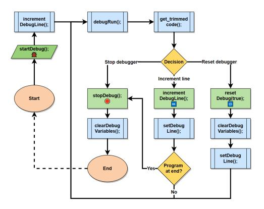
Figure 17: Flow chart for the execution control. The green squares represent calling functions connected to front-end buttons. The blue squares represent called functions.
